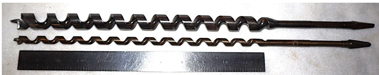
14. Irwin single twist long auger bits.
