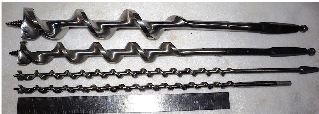
14. Irwin single twist long auger bits.
